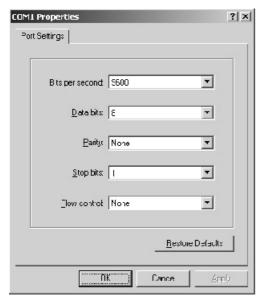
Figure 4-1 Console configuration
